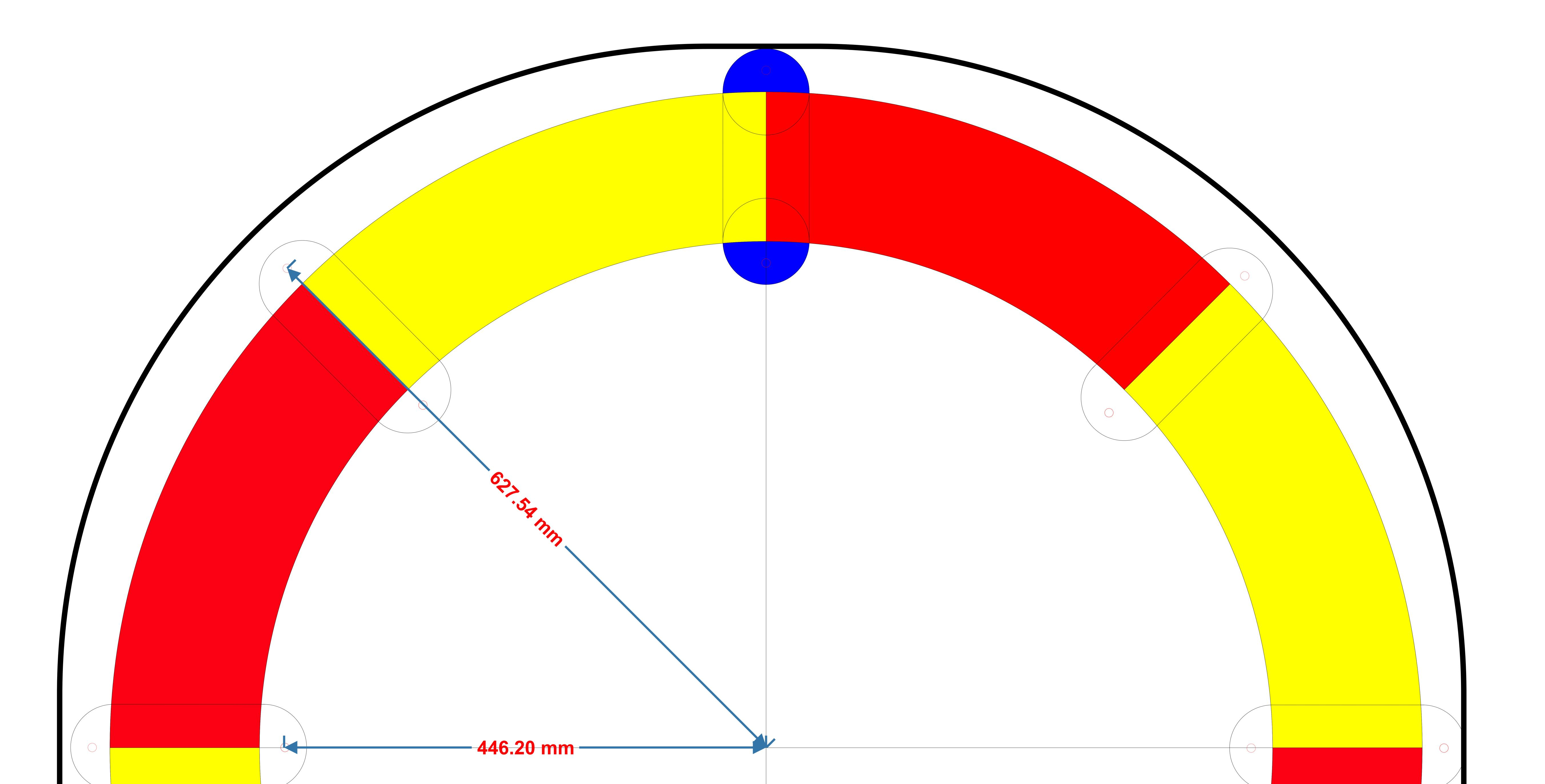
The Rods are M8 so this is a 8mm Hole The outside rods are at 627.54mm Radius The inside rods are at 446.20mm Radius This PDF is at 1:1 scale so if you print it up would be a template to the right size.
